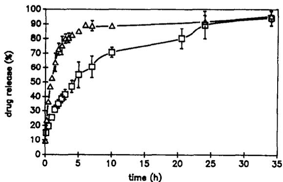
Fig. 7. Percent drug release as a function of time from freeze-dried ( $\square$ ) and air-dried ( $\Delta$ ) hydrogels in simulated gastric fluid without pepsin at 37°C. The absence of an error bar indicates that the standard deviation of the data was smaller than the size of the symbol ( $n=3$ ).
