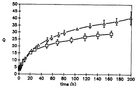
Fig. 4. Swelling kinetics of freeze-dried (□) and air-dried (△) hydrogels in the presence of pepsin. The absence of an error bar indicates that the standard deviation of the data was smaller than the size of the symbol ( $n=4$ ).
