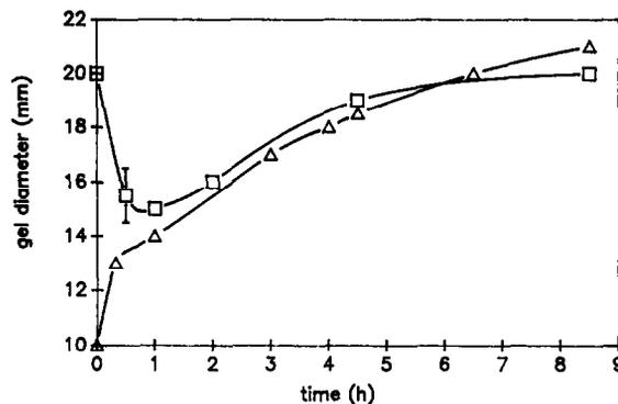
Fig. 2. Dynamic changes in gel diameter of freeze-dried (□) and air-dried (Δ) hydrogels resulting from solvent absorption. The absence of an error bar indicates that the standard deviation of the data was smaller than the size of the symbol ( $n=4$ ).
