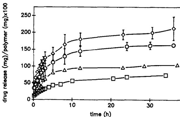
Fig. 8. Drug release from freeze-dried hydrogels as a function of time in simulated gastric fluid without pepsin at 37°C.  $\square$ , one loading cycle;  $\Delta$ , two loading cycles;  $\circ$ , three loading cycles;  $\diamond$ , four loading cycles. The absence of an error bar indicates that the standard deviation of the data was smaller than the size of the symbol ( $n=3$ ).
