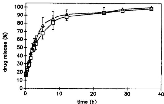
Fig. 9. Percent drug release as a function of time from freeze-dried hydrogels in the absence of pepsin ( $\Delta$ ) and in the presence of pepsin ( $\square$ ). The absence of an error bar indicates that the standard deviation of the data was smaller than the size of the symbol ( $n=3$ ).
