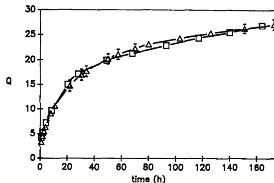
Fig. 1. Swelling kinetics of freeze-dried (□) and air-dried (Δ) hydrogels in simulated gastric fluid without pepsin at 37°C. The absence of an error bar indicates that the standard deviation of the data was smaller than the size of the symbol ( $n=4$ ).
