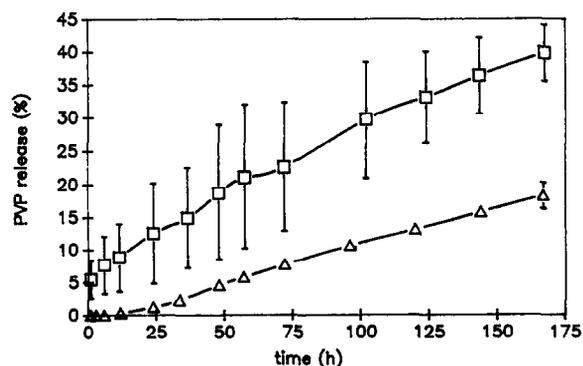
Fig. 3. Release of PVP as a function of time from freeze-dried (□) and air-dried (△) hydrogels in the presence of pepsin. The absence of an error bar indicates that the standard deviation of the data was smaller than the size of the symbol ( $n=4$ ).
